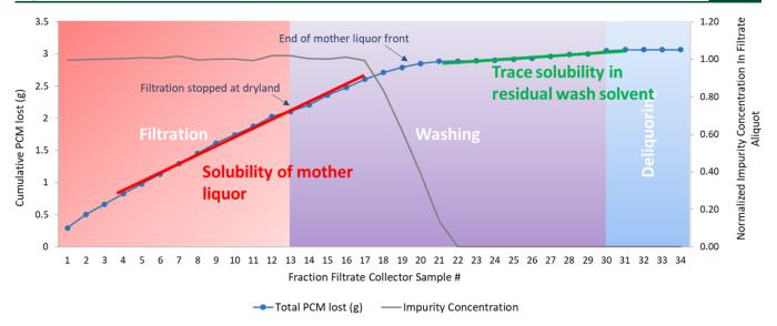
Figure 7. Experiment 1: PCM grade — crystalline, crystallization solvent — ethanol, wash solvent — n-heptane, filtration and washing rate — 10 rpm, volume of wash solvent — 1 cake void volume, number of washes — 3, mass of PCM API lost during wash = 0.1 g
