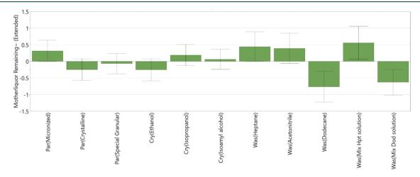
Figure 9. DoE variables that affect mother liquor removal during the wash process;  $R^2 = 0.77$ ,  $Q^2 = 0.27$ , and reproducibility = 0.80.
