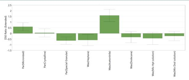
Figure 13. DoE variables that affect PSD  $(D_{50})$  of washed cake — change in  $D_{50}$ ;  $R^2 = 0.82$ ,  $Q^2 = 0.58$ , and reproducibility = 0.97.
