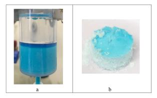
**Figure 11.** (a) Biotage filter tube from experiment 3 after *n*-dodecane wash solvent addition. (b) PCM API cake obtained at the end of experiment 3 with a layer of the blue dye at the top of the washed cake.
