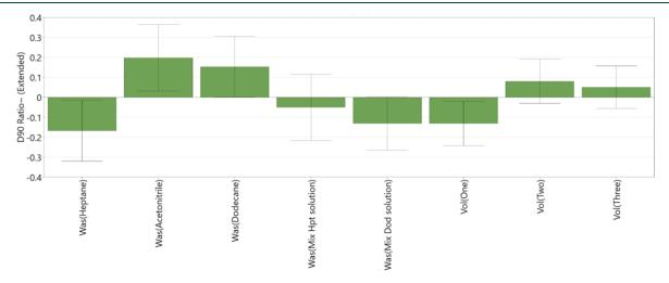
Figure 14. DoE variables that affect PSD  $(D_{90})$  of washed cake — change in  $D_{90}$ ;  $R^2 = 0.60$ ,  $Q^2 = 0.05$ , and reproducibility = 0.81.
