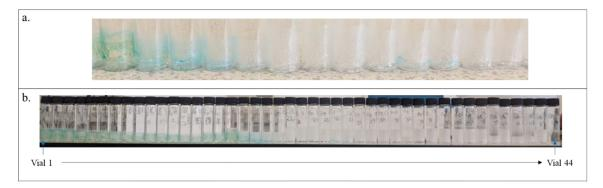
Figure 5. (a) Close-up of a few dried filtrate vials showing the presence of the precipitated material. (b) Collected filtrate vials from experiment 15 showing gradual blue dye impurity removal from the system.
