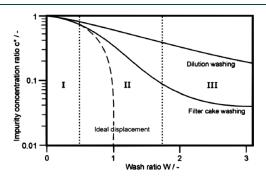
**Figure 1.** Wash curve obtained from measuring the solute concentration of the filtrate. <sup>20</sup> [Reproduced with permission from reference 5160391414737, Copyright 2007, Elsevier].
