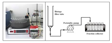
Figure 3. Experimental setup for constant rate filtration, including the process flow diagram of the setup used.
