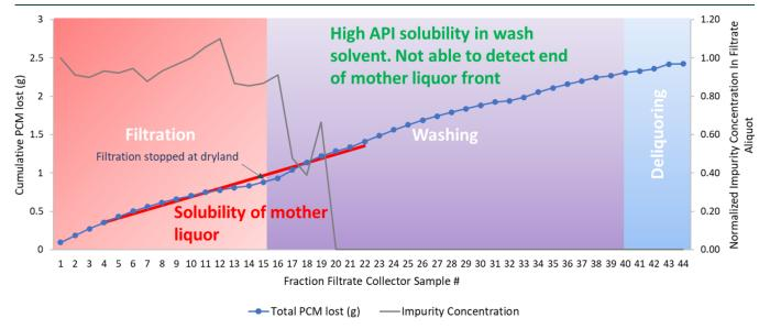
Figure 6. Experiment 15: PCM grade — crystalline, crystallization solvent — isoamyl alcohol, wash solvent — acetonitrile, filtration and washing rate — 100 rpm, volume of wash solvent — 3 cake void volume, number of washes — 3, mass of PCM API lost during wash = 1.48 g.
