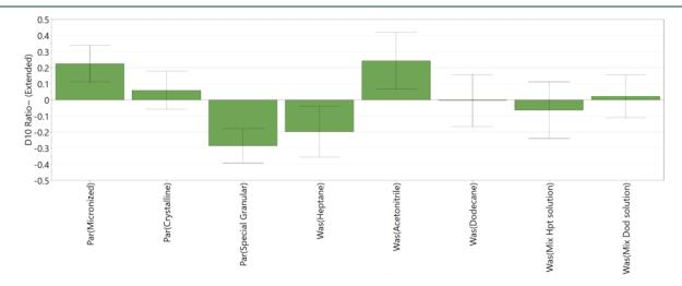
Figure 12. DoE variables that affect the PSD  $(D_{10})$  of washed cake — change in  $D_{10}$ ;  $R^2 = 0.80$ ,  $Q^2 = 0.52$ , and reproducibility = 0.97.
