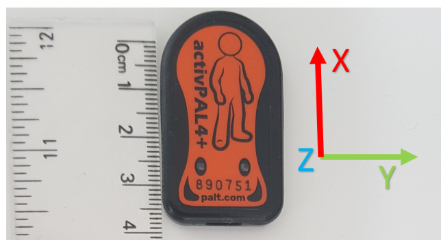
Figure 1. Scaled diagram of an ActivPAL device, with axes of orientation for reference.
