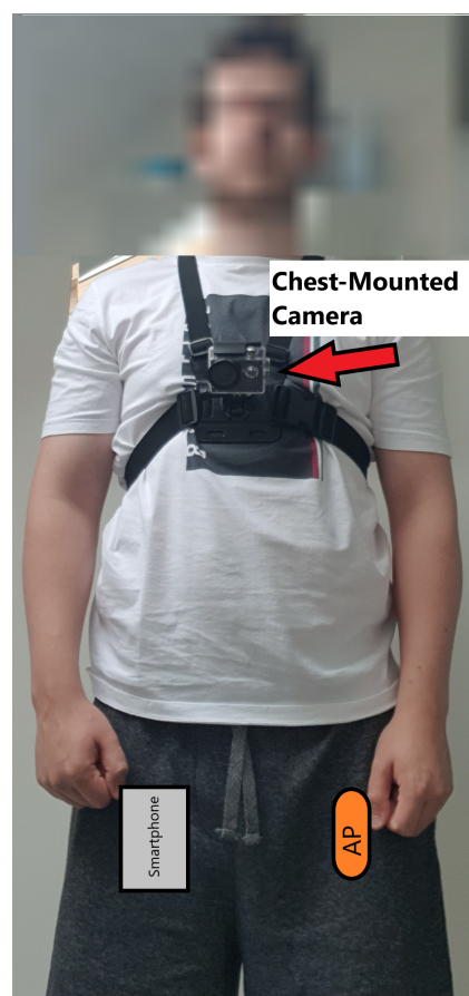
Figure 2. Example of a recording set-up. AP = ActivPAL. The smartphone and ActivPAL would both be worn under clothing.
