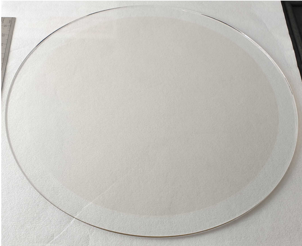
Figure 2. A 1 mm thick, 200 mm diameter glass wafer, coated with a 163 mm diameter Indium Tin Oxide (ITO) electrode on both the top and bottom faces.
