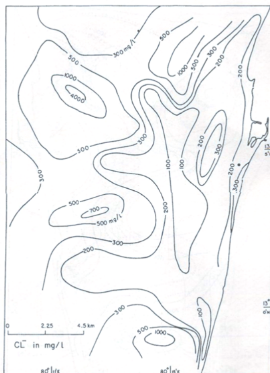
Figure 47. Concentration of chloride ions in groundwater samples represented by isopleth contours at the scale of the city. Ballukraya and Ravi. 513
