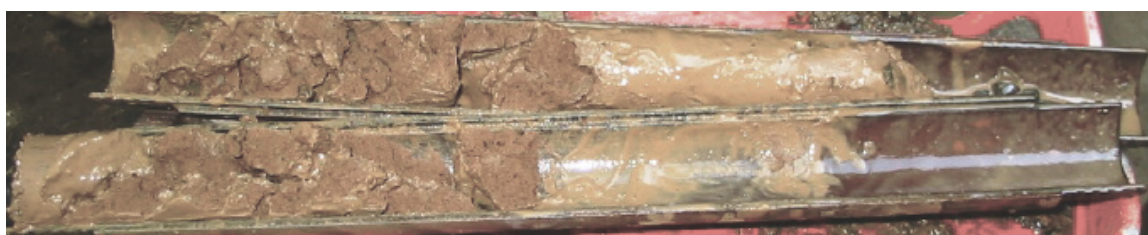
Figure 36. Disturbed soil sample. Systra/IGS. 401
