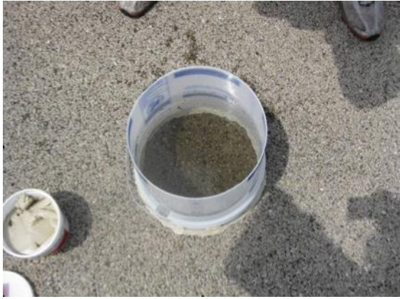
Figure 6: Infiltrometer at Permeable Pavement at St. Margaret Mary Parish
