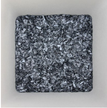
Figure 6.5.: Seeding layer of fine polysilicon chunks placed on the bottom of G1 crucible for the growth of an HPM ingot.
