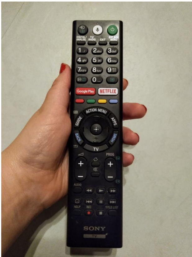
Figure 1. Modern remote Controller. Arrow keys that are often used for moving inside smart applications can be found in the middle of the controller. T9 keyboard is located on the upper part of the controller.
