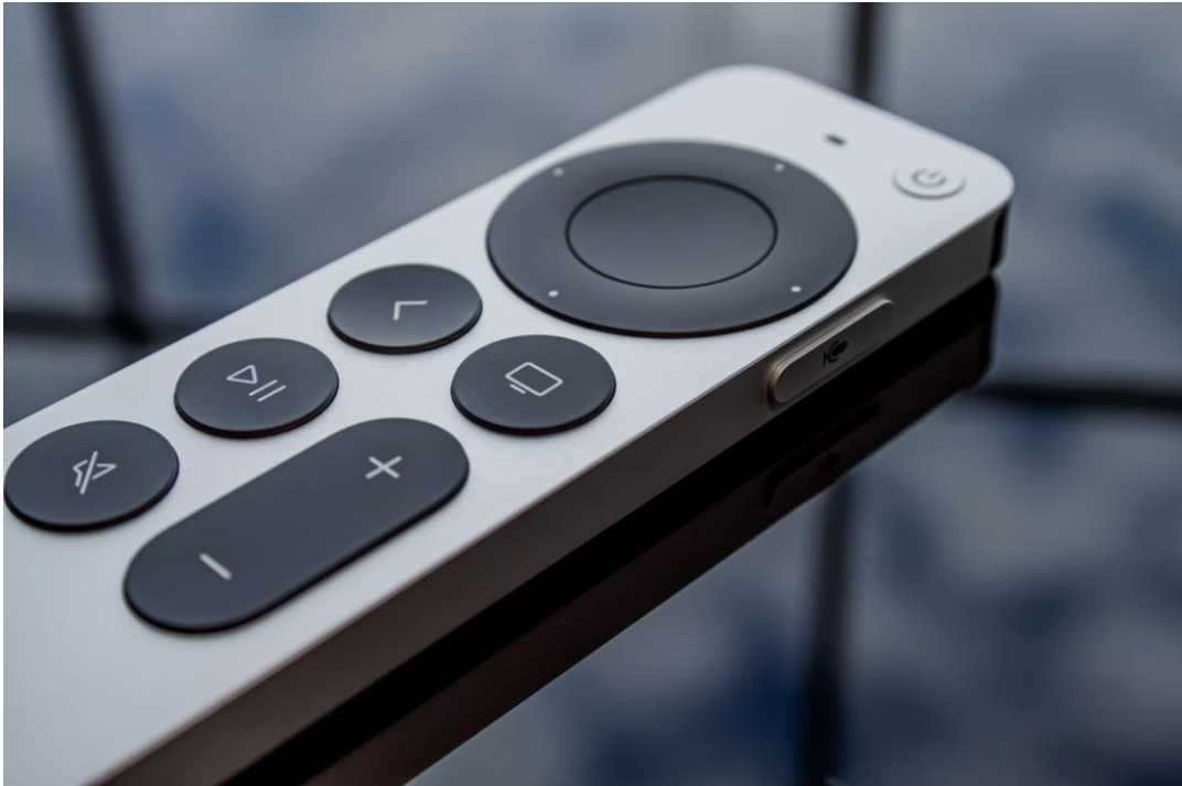
Figure 2. Apple TV Remote Controller. Apple has decided to minimize the number of buttons by creating a simple remote controller. (Picture by Yarema, Unsplash (2021)).
