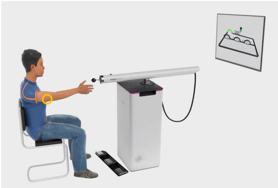
Figure 2.1. The experimental setup. The participant is seated in front of the LCD screen, at reaching distance from the sensor of the HM. The electrodes for delivering electrical stimuli, are placed on the triceps tendon of the right arm (yellow circle), and the triple foot switch is used to give pain-related fear and pain-expectancy ratings. Figure modified with permission from Glogan, Gatzounis, Vandael, et al. (2020).
