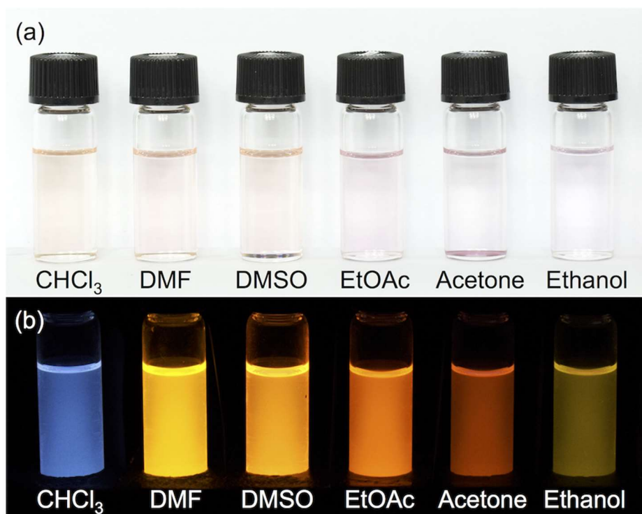
Figure 4.1.2.2: Ant10-T 8 W 2 nanoparticles dispersed in different organic solvents (5.0 mgml -1 ): (a) Under normal light, (b) excited at 365 nm. EtOAc: ethyl acetate.
