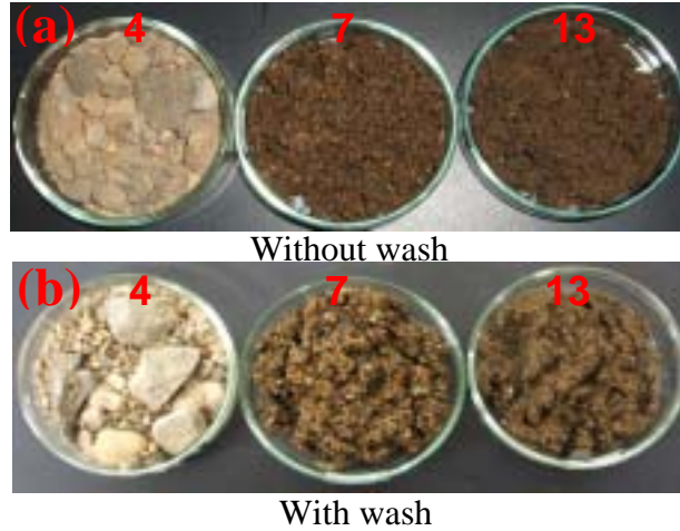
Fig. 3-1. Sediment samples without wash a) and with wash sieving on 80-mesh b).
