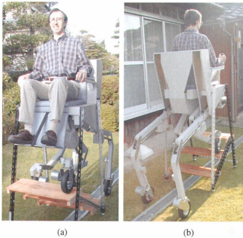
Fig. 78 Third proposed mechanism modeled with electric actuators – stair-climbing mode
