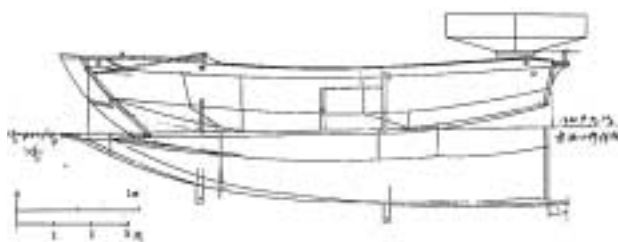
図2-2 和船板図の一例 長崎市京泊, 清水直治氏図面, 昭和45年10月作製の釣船 A hull diagram of a Japanese style fishing boat "wasen", which is drawn on a wooden plate by N. Shimizu, a boat-builder in Nagasaki.
