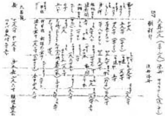
図2-7 田島弥三による和船寸法書の例 The various dimensions of hull diagram for building a Japanese style of fishing boat “wasen” of 9.6m in length, written by Y. Tajima in Tara, Saga Prefecture during the Showa period.
