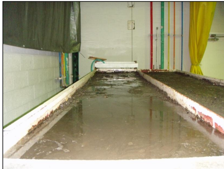
Figure 4.3 Experimental set up to study erosion pattern from overland flow.
