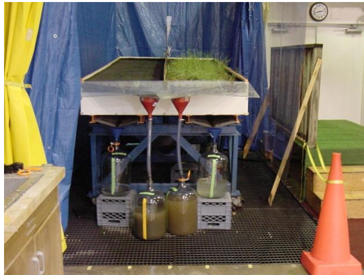
Figure 4.1 Tilting soil chamber with surface and subsurface sample collection systems (Trask, 2002).
