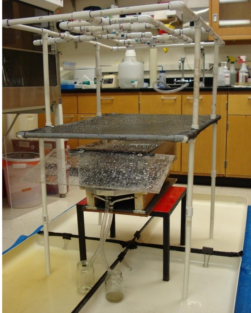
Figure 4.2 Complete laboratory-scale rainfall simulator and tilting soil bed system (Davidson, 2010).
