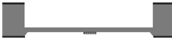
(c) Sputter deposit 100 nm aluminum
