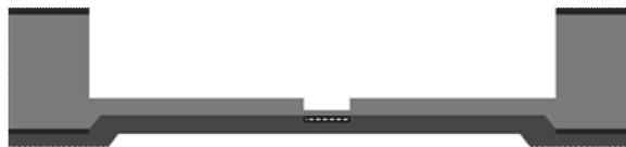
(e) Sputtering deposit 100 nm silver and 300 nm copper
