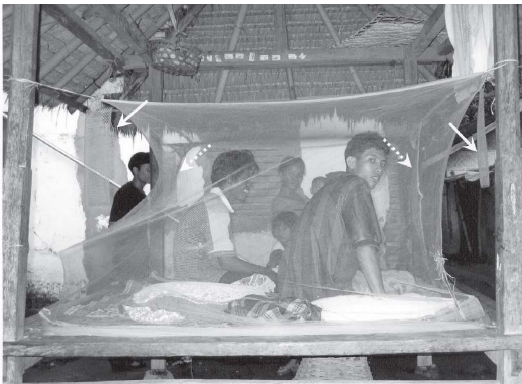
Figure 2. Field test with four plastic strips in a beruga . Arrows indicate the plastic strips treated.
