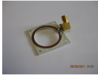
Figure 8.4: Microwave coil machined from the material Rogers Corp. R04350B with a soldered SMA connector.
