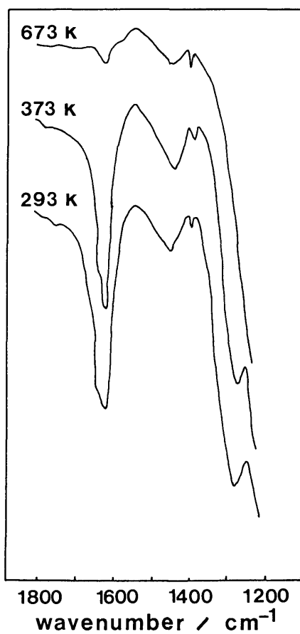
Fig. 10. IR spectra for CuY during NH 3 treatment.
