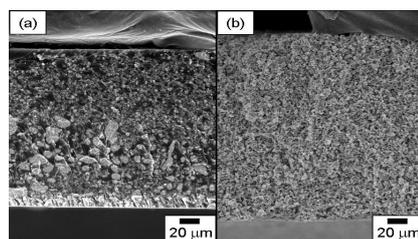
Fig. 1. SEM images of cross-section of Cs-PWA-dispersed membranes, which employed (a) Epicoat 828 and (b) E201 as matrices.
