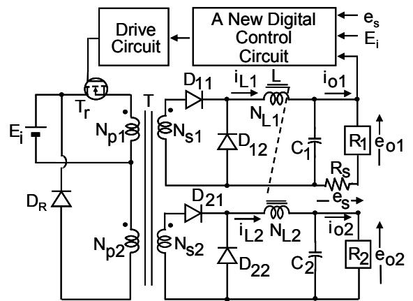
Fig. 1 A new digital control multiple-output dc-dc converter.
