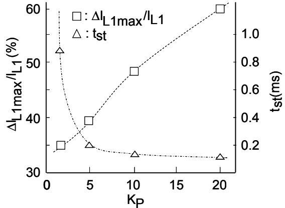
Fig. 6 Relationship among transient time  $t_{st}$  of the output voltage, overshoot of the reactor current and the proportional coefficient  $K_p$  of the moving average.  $K_I=0.024$  and  $K_D=2$ .
