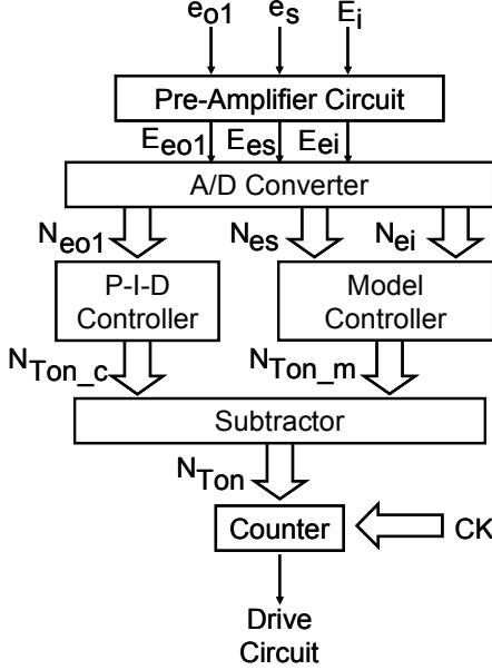
Fig. 2 A new digital control circuit.
