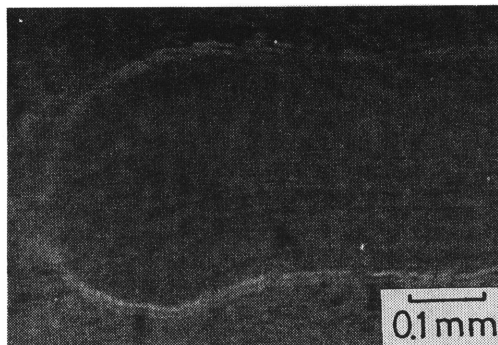
(B) The trace on a flat surface which shows a contact width at beginning
