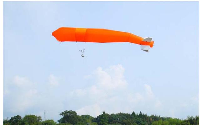
Fig. 15. Balloon type flying robot.
