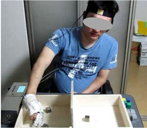
Fig.14 Pick and place test using assistive glove
