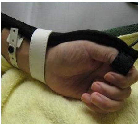
Fig.10 Bending sensor attaché to thumb finger
