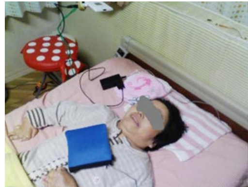
Fig.7 Flat type capacitance switch on the chest
