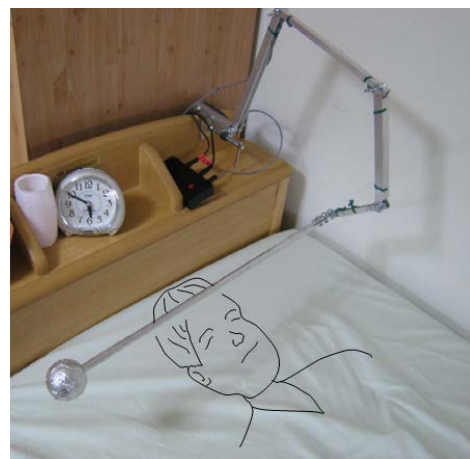
Fig.4 Rod type touch switch
