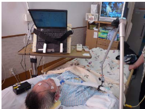
Fig.14 Input device to use EOG signal
