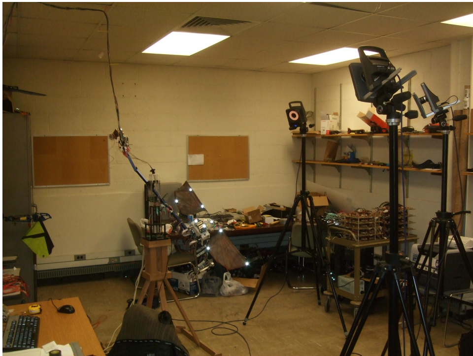
Figure 4.18: Vicon cameras around robotic bat
