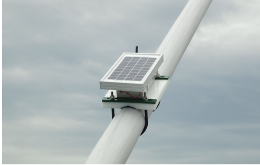
Figure 9.11: Solar-powered sensor node attached to a bridge cable.
