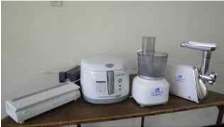
Fig. 2: Micro processing system for fish paste processing (from left, vacuum sealer, deep fryer, food processor, mincer)
