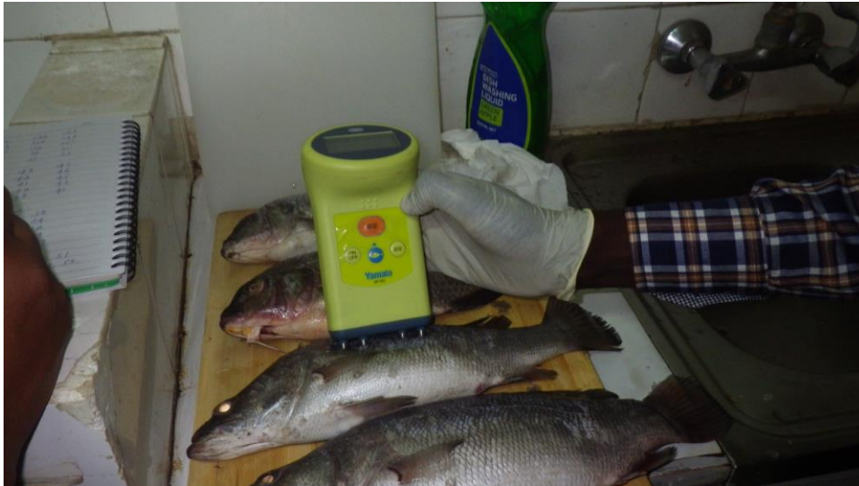
Figure 8: Measurement of impedance using the portable device
