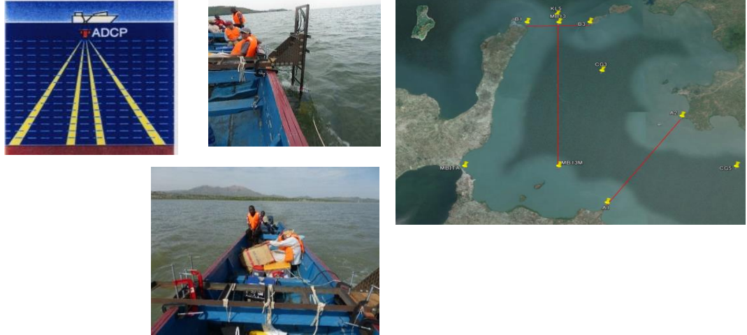
Fig. 2 Monitoring Flow Current at the mouth of Nyanza Gulf using ADCP
