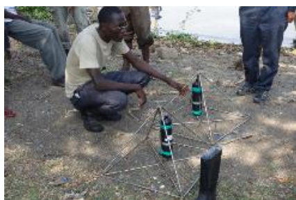
Fig. 10. Acoustic receivers set in the Lake
