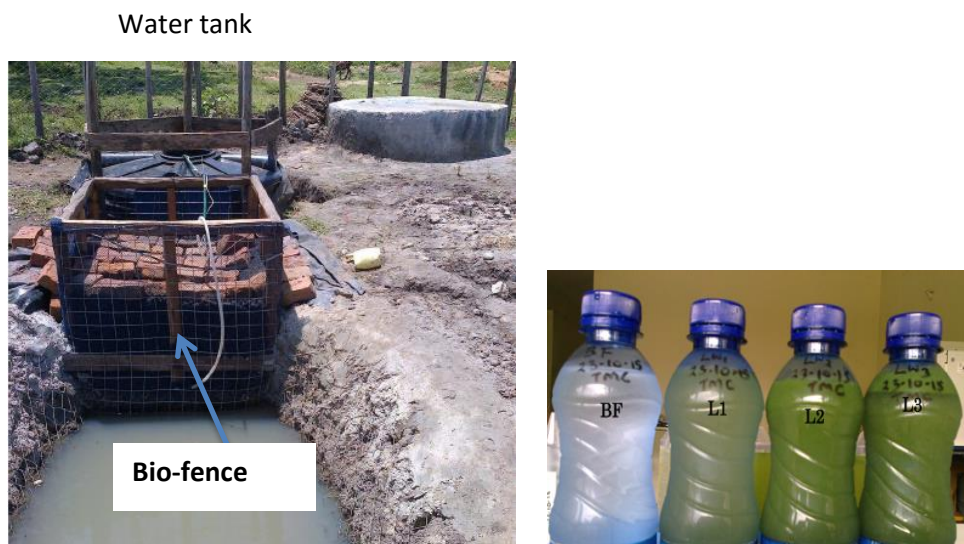
Figure 4. The photograph of the constructed fixed type Bio-fence at Ogal beach. Left side photographs of waters in plastic bottles shows a typical treatment effect by this Biofence (October/2015), where BF shows the treated water by Biofence, then L1, L2, L3 show the outside lake water at several places near Biofence.
