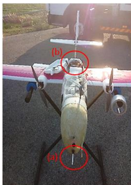
Figure 12. The integration of POPS OPC in the I-SOAR fixed-wing UAV. Circle (a) shows the inlet placed at the front of the UAV, and circle (b) shows the instrument installed inside the UAV.
