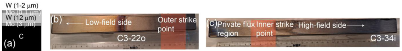
Figure 3. (a) Schematic illustration of the produced layer configuration on the marker tiles exposed during the WEST C3 and C4 campaigns. ((b) and (c)) Photographs of two marker tiles removed from the (b) outer (tile C3-22o) and (c) inner (tile C3-34i) divertors of WEST after its C3 campaign.
