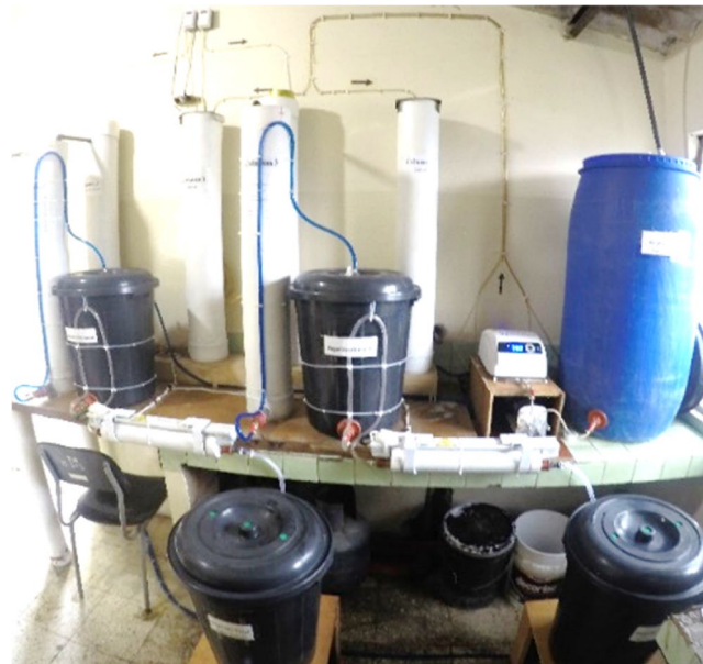
Fig. 1 Pilot plant to purify rainwater at a single-family level in the rural sector, with a capacity to purify 50 L/day
