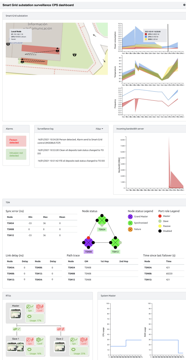
Fig. 4 Final CPS dashboard: Monitoring information is displayed for each of the subsystems (top: video surveillance; middle: TSN; bottom: smart grid monitoring and control), as well as hardware information for the different platforms. As can be observed, depending on the type and nature of the information to be represented, a different kind of representation is used: Numerical data that require their evolution over time are represented in line charts or scatter plots. Data whose importance is limited to the moment it is generated is displayed as a KPI with its own value. Data that is relevant because it has already been processed is shown in a text log.
