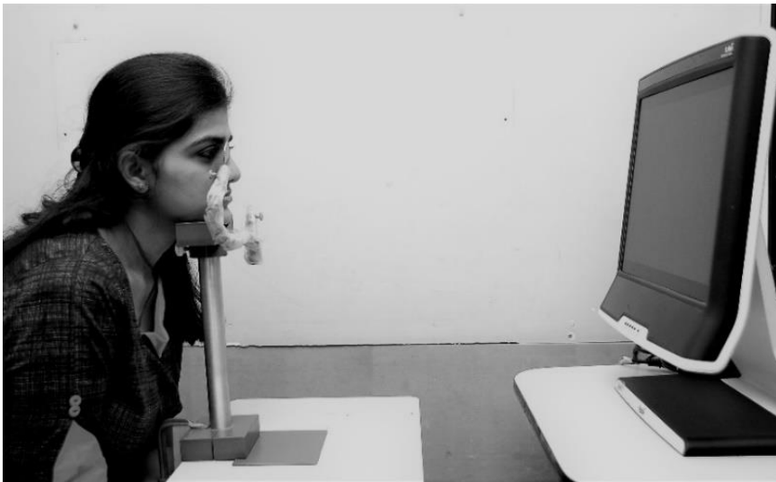
Figure 3.1. EMP test set up comprising of a 17-in TFT monitor with an inbuilt infrared-based eye-tracking camera at the bottom panel. The chin rest placed at a distance of 55 cm was used for each measurement including a PMMA blocker holder positioned in a standard lens holder.
