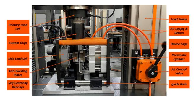
FIGURE 1. Anti-buckling device mounted onto a universal load frame.
