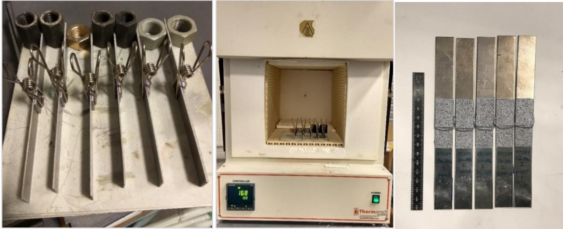
Figure 10. Process used for producing Stress-free adhesive-bonded single lap shear specimens
