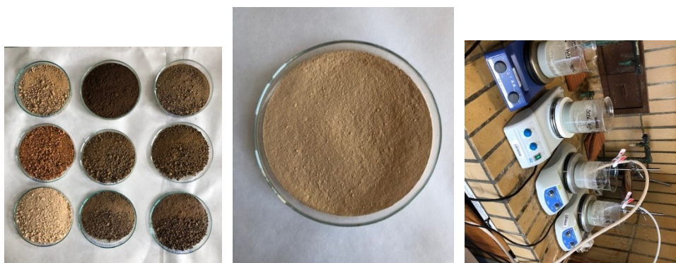
Figure 1 Preparation of samples for leaching and the leaching process. Source: (own)
