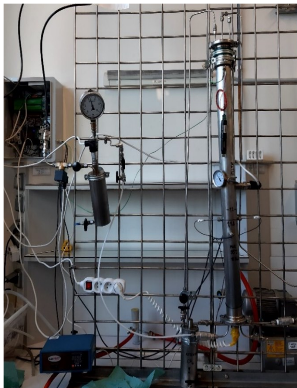
Figure 2 Photo of biogas purification apparatus. Source: (own)
