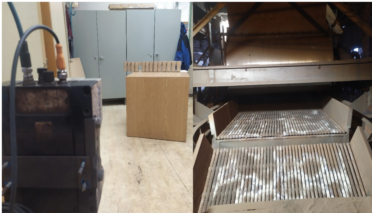
Figure 2 Model of individual rods and sintering carts. Source: (own)
