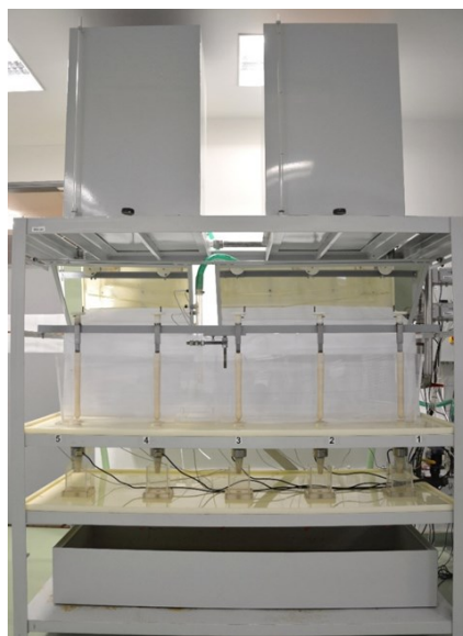
Figure 1 The Physical model of five-strand tundish with accessories. Source: (own)
