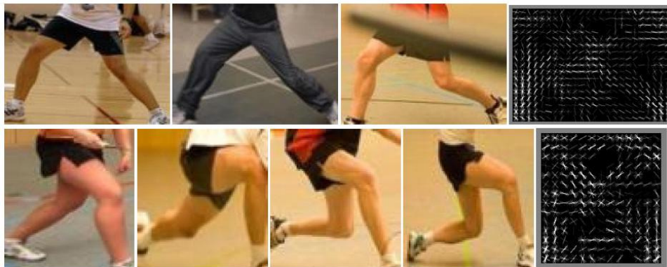
Figure 4.1. Examples of two poselets of the part legs. Each row are patches of the same poselet. The last column is the HOG templates of the poselets. This figure is from Wang et al. [57].
