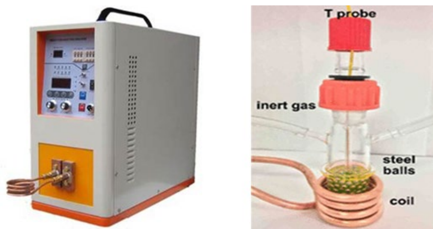
Figure 2.5 (A) Inductive heater used in this dissertation and (B) The reactor setup in the IH system.
