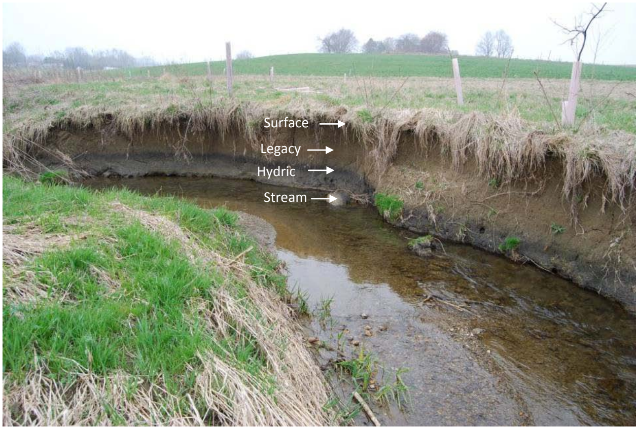
Figure 3.2. Picture of current altered environmental conditions at BSR. Bottom dark layer represents relict hydric sediments from a former wetland. Lighter top sediments are depositional legacy soils from ponding. Soils are labeled to represent where the 4 strata were collected. The surface and legacy sediments will be removed in the restoration.
