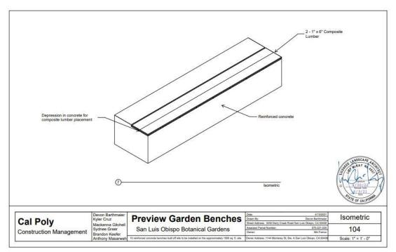
Figure D – Isometric
