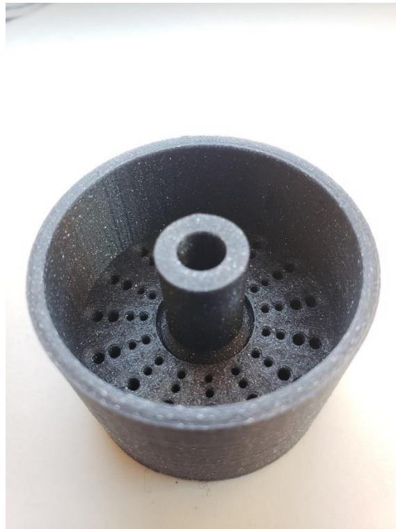
Figure 33. Porous Design 3D printed structural Design.
