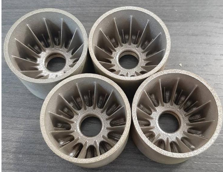
Figure 58. AM printed Alloy X Fin Design by Solar Turbines.
