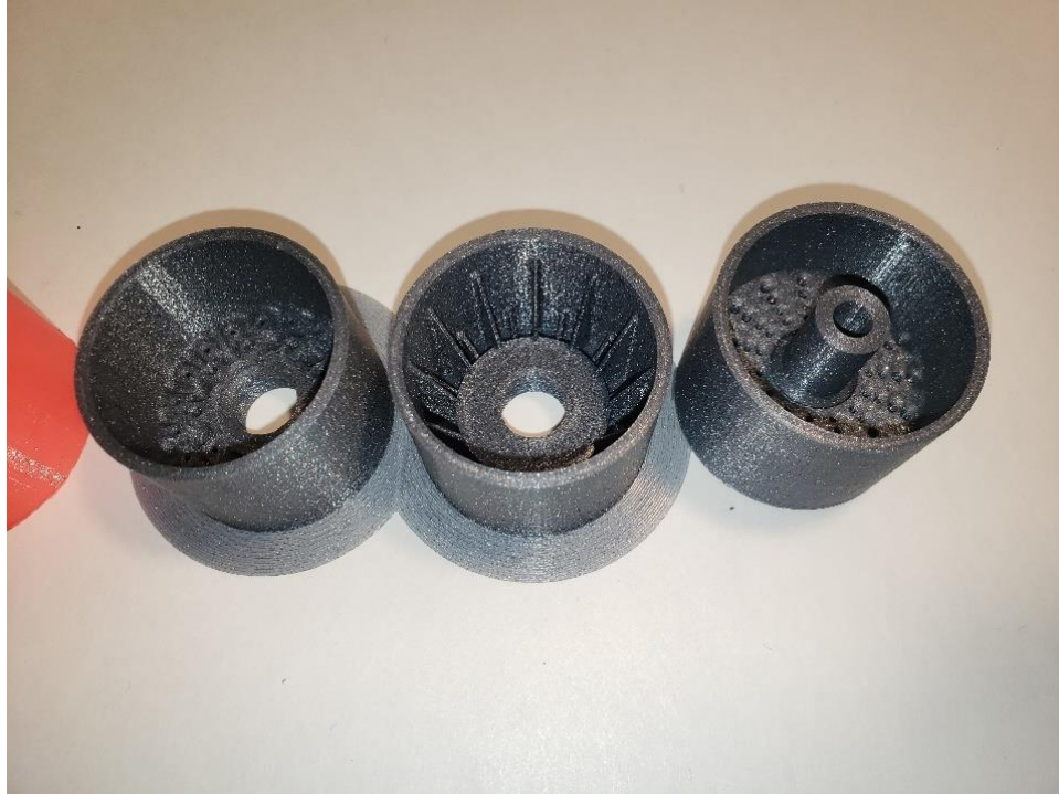
Figure 32. Structural prototypes 3D printed from plastic.
