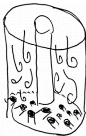
Figure 17. Porous structure for turbulent airflow.
