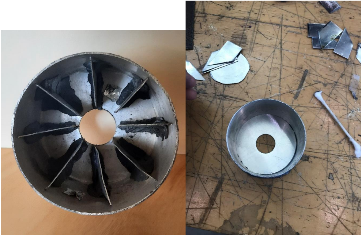
Figure 57. The simplified Fin Design (left) and the Flat-Plate (right) for a comparative heat test.
