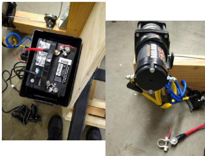
Figure 2: Battery and Winch Connections for operation
