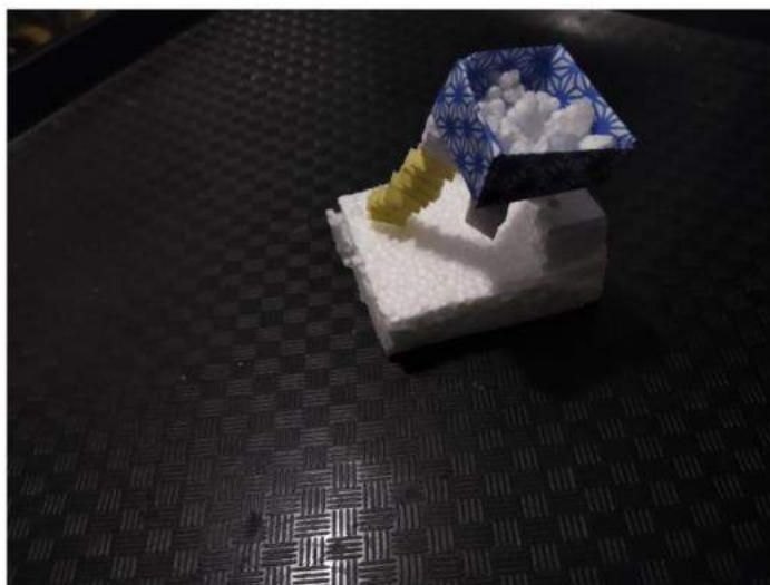
(Above) 1. A gaylords tilter with the support beams across the diagonals of the box. The tilter stays at one height at one corner, and tilts the other corner to various heights to tip the produce within the box.
