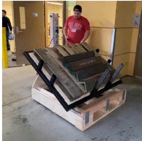
Figure 40. Drilling Screws into Bottom of Base System
