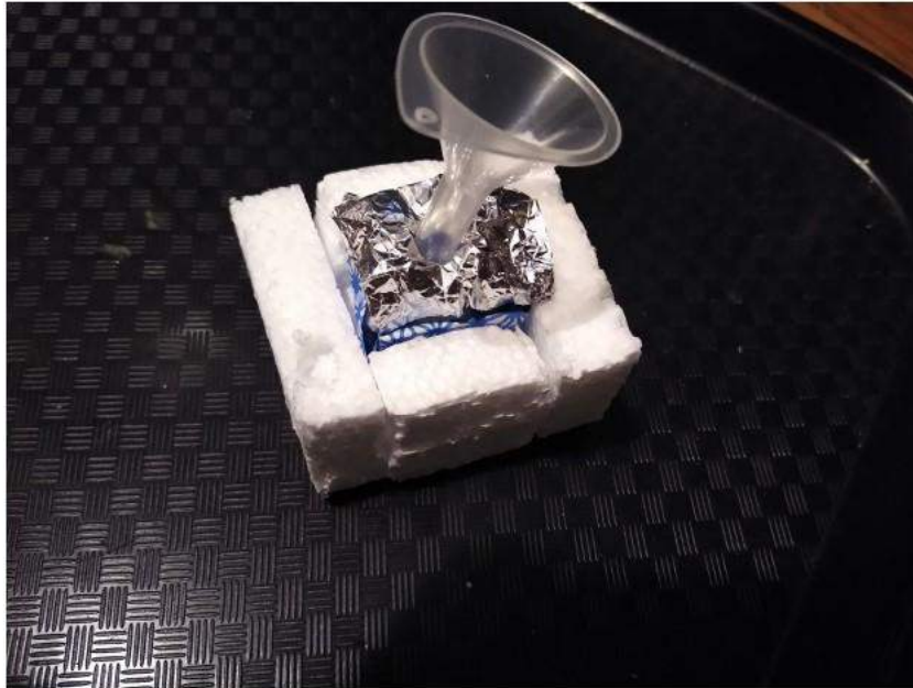
(Above) 5. The gaylords box is covered from above, with a vacuum pump attached above to vacuum the produce from within the box. Alternatively, the pump could be pushing air in to push produce out from another hole elsewhere.
