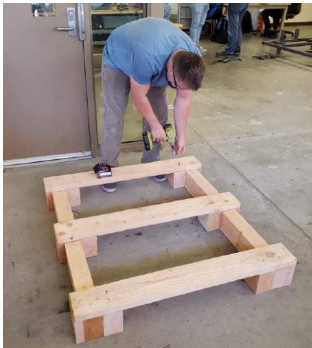
Figure 38. Drilling Screws into Bottom of Base System
