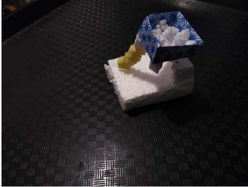
(Above) 1. A gaylords tilter with the support beams across the diagonals of the box. The tilter stays at one height at one corner, and tilts the other corner to various heights to tip the produce within the box.
