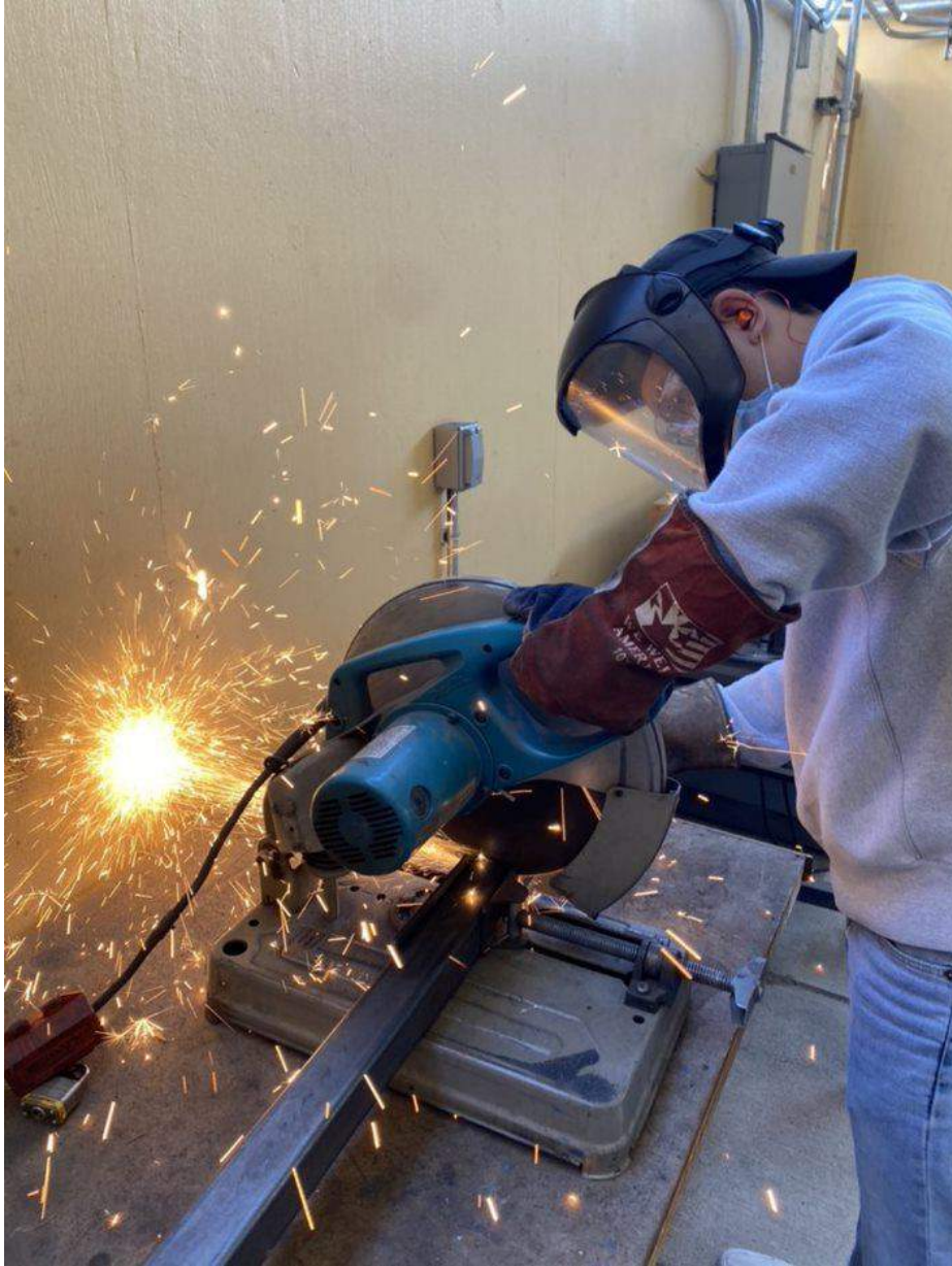
Figure 33. Cutting Steel Tube with Abrasive Saw
