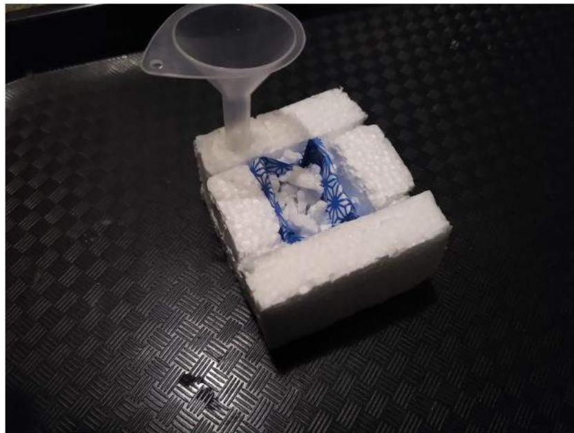
(Above) 4. An enclosure around the box, where the enclosure is filled with salt water so that the produce floats inside.
