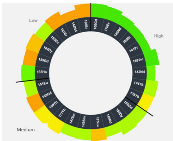
Figure 17. DVS panel designer. Each channel tile is arrayed counterclockwise on the wheel in order of ascending tolerance values: low, medium, or high. The channel tile height is proportional to the sensitivity area of the machine (optimal delivery of metals in 153-176). The tile is heat-mapped (green-orange) to indicate the signal overlap into the channel (% of tolerance value for the target in that channel). Printed with permission from Fluidigm.
