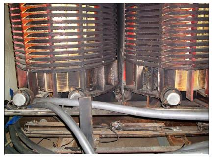
Figure 2. Insulation system failure due to contamination
