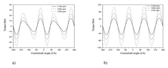
Figure 7. Variation of mass torque; a) individual cylinder and b) total mass torque.
