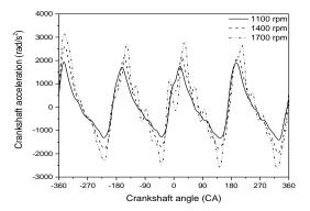
Figure 6. Estimation of instantaneous filtered acceleration of crankshaft.
