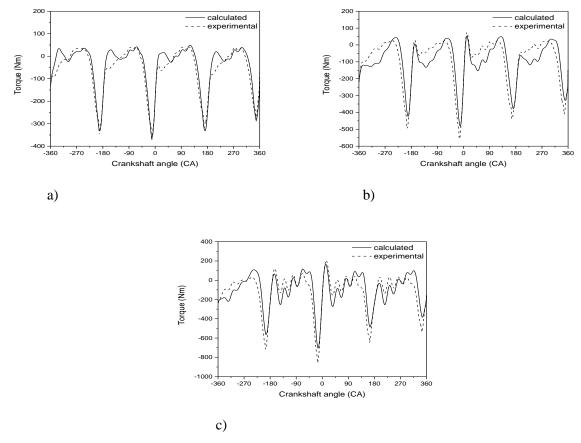
Figure 12. Comparison between measured and predicted of the engine total friction torque.
