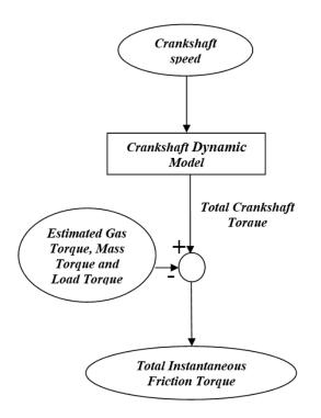
Figure 3. The flowchart of the estimation algorithm.
