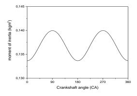
Figure 5. Inertia of the crankshaft assembly.
