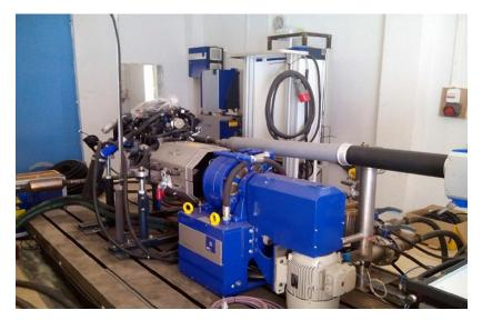
Figure 1. View of the engine test bench [30].
