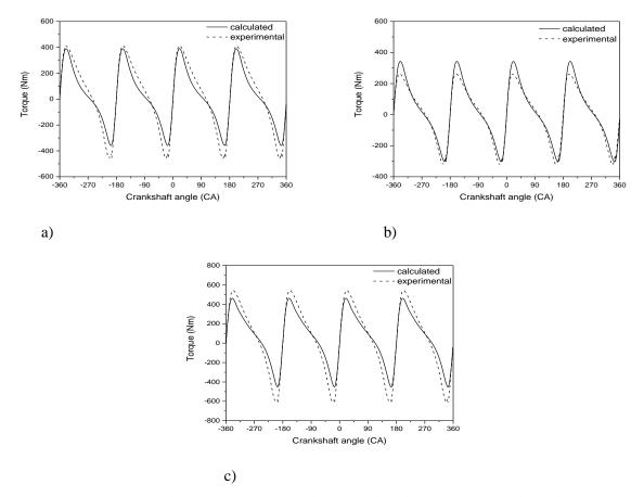
Figure 9. Comparison between measured and predicted of the engine total indicated (gas) torque.
