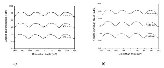
*Figure 4. Instantaneous crankshaft speed: a) measured signal and b) filtered signal.*
