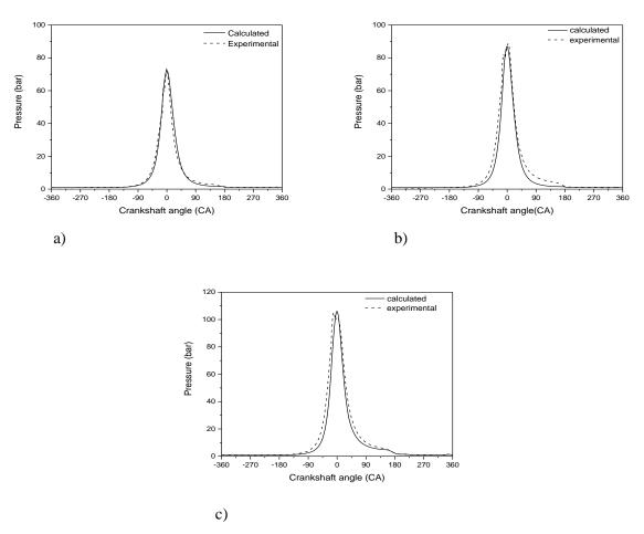
Figure 2. Comparison between measured and simulated in-cylinder pressure.
