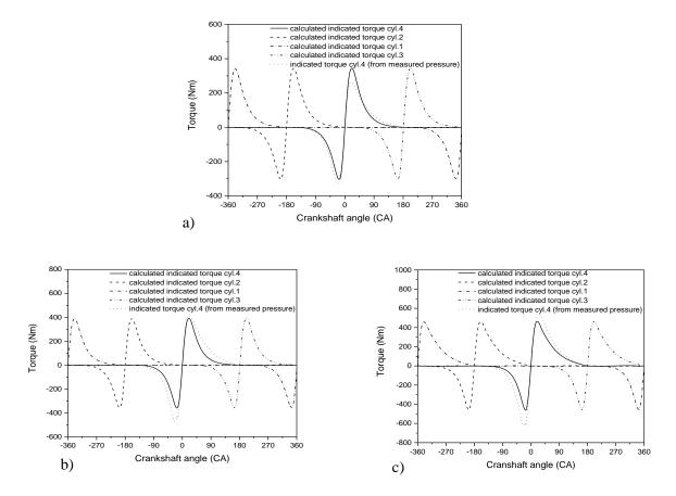
Figure 8. Comparison between measured and predicted gas torque for the fourth cylinder.
