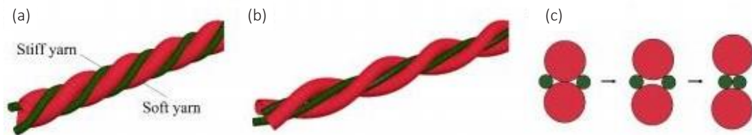
Figure 6. 4-ply auxetic yarn: (a) at rest; (b) under extension; and (c) cross-section views at different stages of stretching [2]
