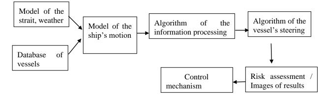
Fig. 2 Block diagram of an automated control system
