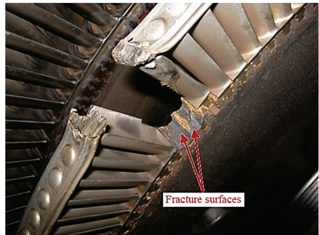
Figure 1 Example of rotor blade fracture [3]
