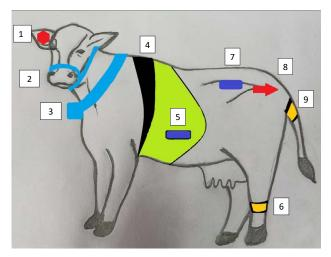
**Figrue 1.** Proposed engineered devices in a dairy cow for continuous observation of well-being status: (1) ear tag, (2) halter, (3) neck collar, (4) automatic blood sampler, (5) reticulo-rumen bolus, (6) pedometer, (7) vaginal bolus, (8) tail-head chip, (9) upper tail ring.
