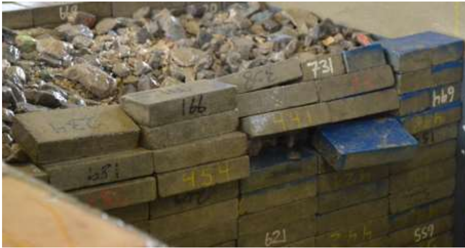
Figure 7.23 Series 4, progressive damage to front wall following partial loss of fill
