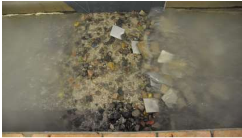
Figure 7.33 Series 6, leeward wall post failure
