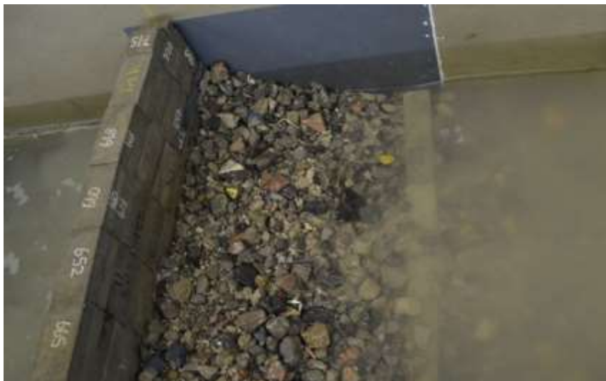
Figure 7.24 Rear face following failure of front face, Series 4
