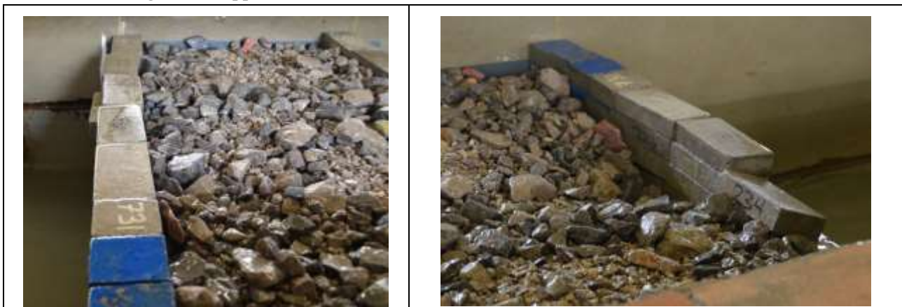
Figure 7.22 Series 4, start of damage with sink-hole in fill following loss of front face blocks
