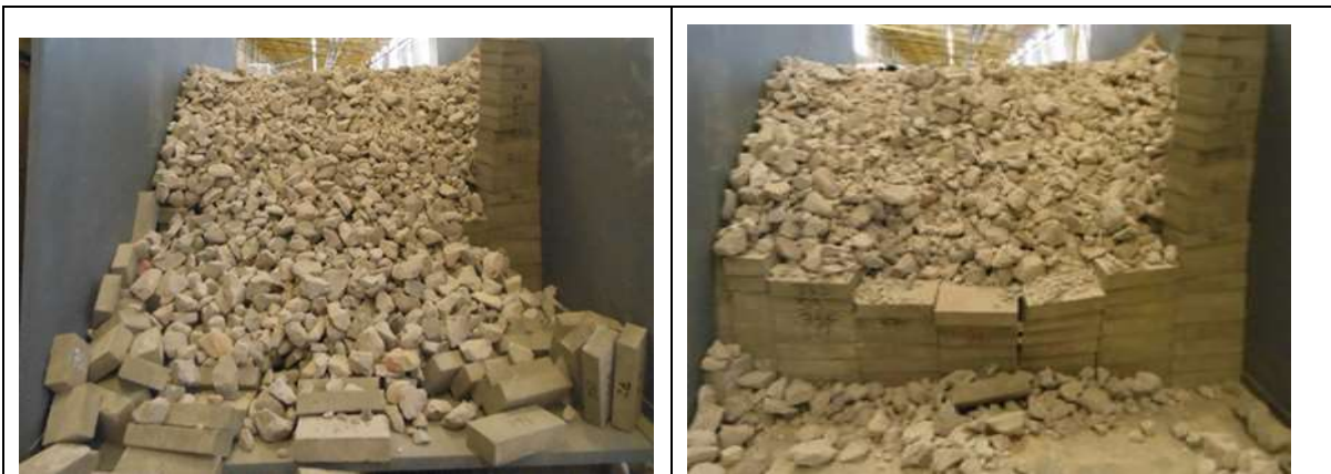
Figure 7.4 Example dry-build failure
