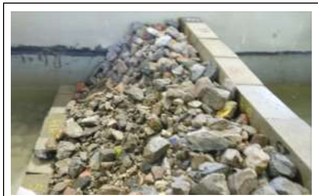
Figure 7.10 Test Series 1, post front wall failure
