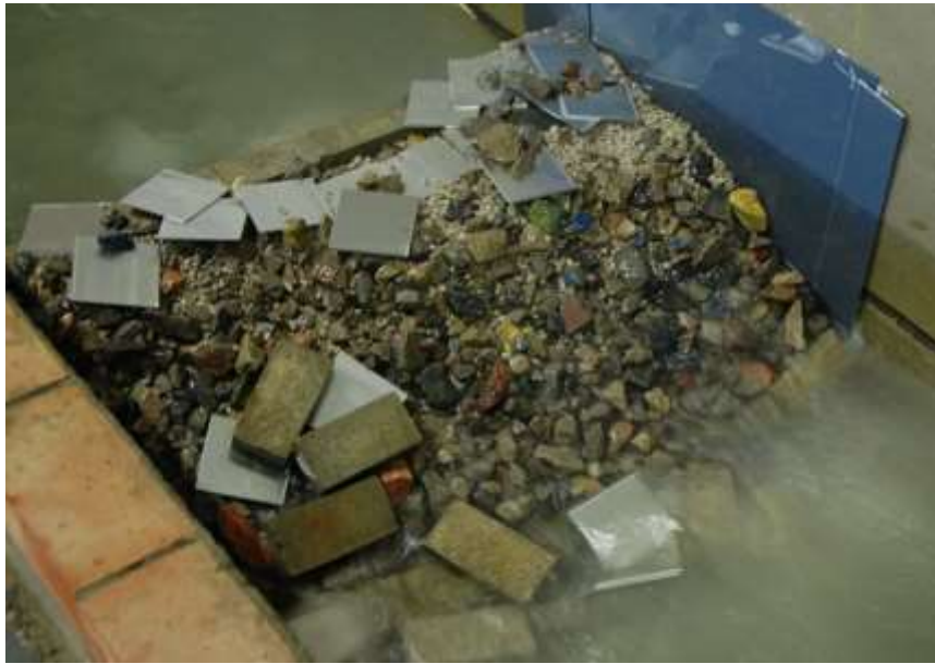
Figure 7.29 Section 5 after collapse of the seaward wall
