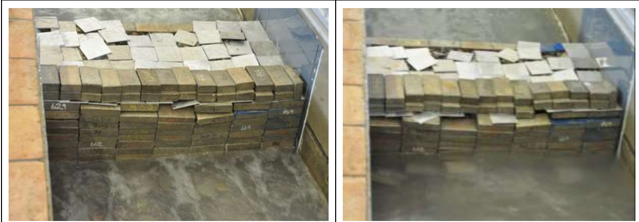
Figure 7.31 Series 6, block extraction on the front face, later damage progression
