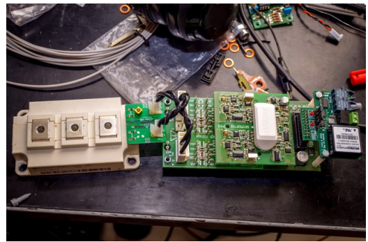
(b) L6100231 SKYPER 32PRO R (Semikron). Si-IGBT driver.
