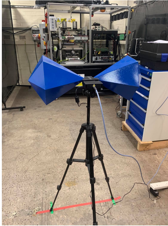
Figure 3.33: BicoLOG 20100 X from Aaronia. Positioned to detect radiated emissions from DPTR.
