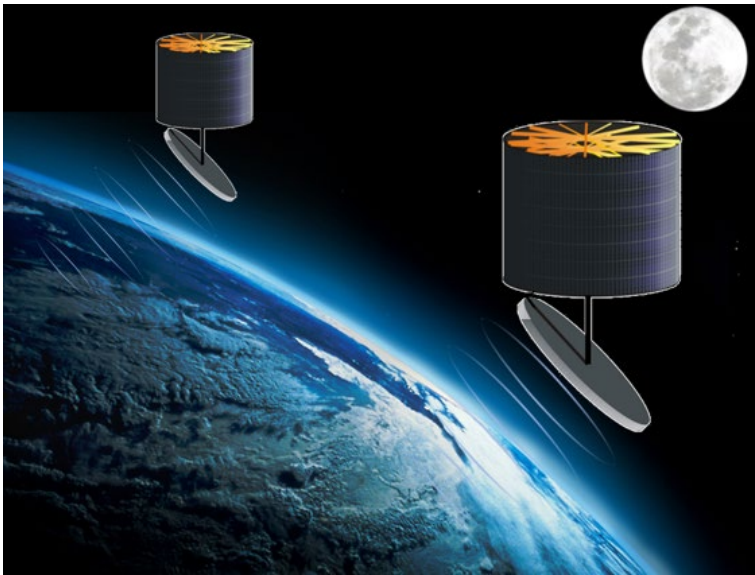
Figure 6: Multiple “Tin Can” solar power satellites in geosynchronous earth orbit beaming power to terrestrial markets.
