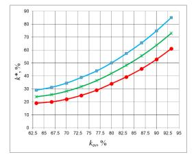
Figure 4. Dependence of the contrast on the overlap coefficient for marking with a CuBr laser for power densities: red colour  $-q_{sl} = 0.99 \times 10^{10} \text{ W/m}^2$ ; green colour  $-q_{s2} = 1.20 \times 10^{10} \text{ W/m}^2$ ; blue colour  $-q_{s3} = 1.42 \times 10^{10} \text{ W/m}^2$ .
