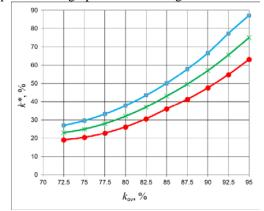
Figure 3. Dependence of the contrast on the overlap coefficient for marking with a fiber laser for power densities: red colour  $-q_{sl} = 1.24 \times 10^{10} \text{ W/m}^2$ ; green colour  $-q_{s2} = 1.50 \times 10^{10} \text{ W/m}^2$ ; blue colour  $-q_{s3} = 1.77 \times 10^{10} \text{ W/m}^2$ .
